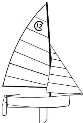
The Cadet Dinghy has gone through an extraordinary number of changes over time: from heavy wooden hull through light-weight Western Red Cedar hull to fibreglass hull, from gaff rig to bermudan rig, from fully open boat with no added buoyancy to fore and aft buoyancy tanks and ultimately to fully integrated side buoyancy tanks, from steel centreplate to aluminium alloy centreplate, and from fixed blade rudder to swing blade rudder.
